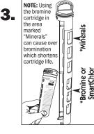
Snap the SPA FROG Mineral Cartridge into the area marked "Minerals" (top portion) and the SPA FROG Bromine Cartridge into the area marked "Bromine or SmartChlor" (bottom portion) making sure to line up the indentation at the top of the cartridges with the raised area on the holder.
