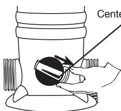
In the back of the Prevail Cycler depress center of locking pin with a finger and pull pin out of dial.
