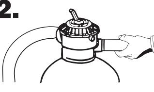
Screw one end of nipple into the filter return.
