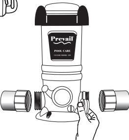
If using **female adapters**, apply pipe thread tape or sealant to the threaded end of each Cyler port.
