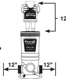
Allow a minimum of 12" above and on each side of Prevail Cyler to ensure room for replacement of Prevail Pool Pack.
