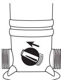
Replace locking pin by pushing it through the slots on the dial until it locks into place.
