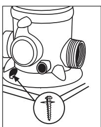
For better stability, Prevail Cyler may be mounted on a treated wood base using **Phillips pan head screws**, one in front and two in back. If you have questions about stability, please contact your dealer or King Technology.
