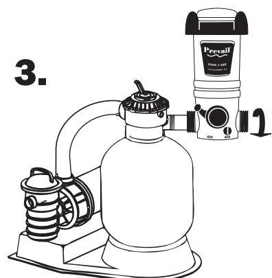
Screw either side of Prevail Cyler on to open nipple end until upright and secure.
