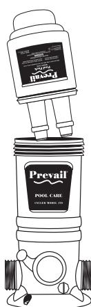
Insert Prevail Pool Pack into Prevail Cyeler, lining up the openings in Prevail Pool Pack with keys in Prevail Cyeler.
