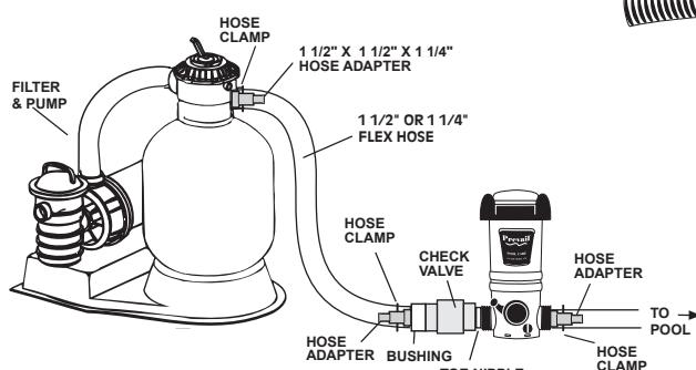
4. To prevent damage to heaters or filters, see your dealer about installing a **corrosion resistant check valve** which will reduce the back flow of chlorine gas when the Cycler is turned off.
