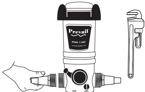
2. Screw adapters into each end of Prevail Cycler. Hand tighten. Finish tightening by turning 1 to 2 revolutions with a pipe wrench. **DO NOT OVER TIGHTEN.**
