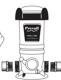
If using **male adapters**, apply pipe thread tape or sealant to the threaded end of each adapter.
