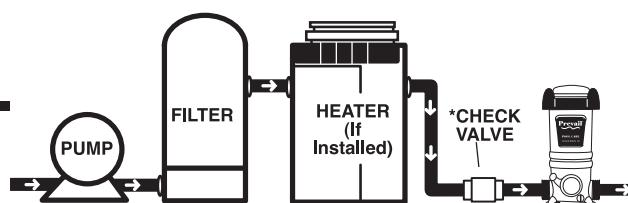
To prevent damage to heaters or filters, see your dealer about installing a **corrosion resistant check valve** which will reduce the back flow of chlorine gas when the Cyler is turned off.
