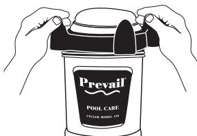
Replace cap by hand only. **DO NOT OVERTIGHTEN.**
