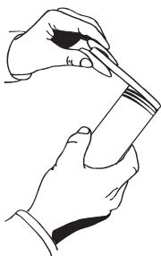
Apply pipe thread tape or sealant to each threaded end of nipple.
