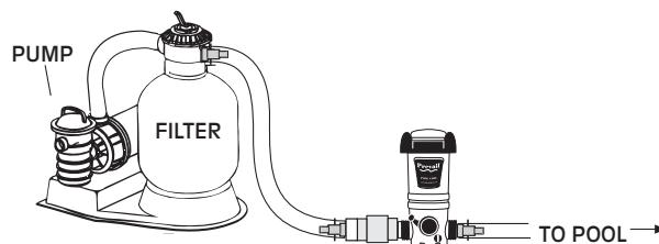
The Prevail Cycler should always be installed between the filter and pool (or between heater and pool if applicable). Never install Prevail Cycler before the heater or damage to the heater could occur.
