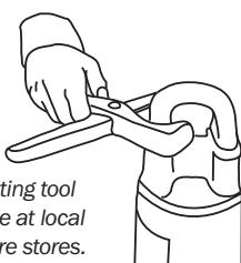
**3B.** Place curved section of tool around the narrow end of one pack tower and line up blade on indent
