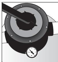
Check the pool's filter gauge often and periodically clean filter per the manufacturer's directions. A dirty filter will slow the flow of water which could hamper proper circulation.
