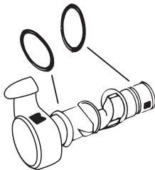
Replace both O-rings. Apply silicone lubricant that came with your Prevail Cycler on O-rings.
