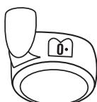
Turn off pump. Turn dial to 0. This reduces the flow of water into the unit when the cap is open.
