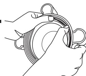
Place your thumbs on each side of the cap over the O-ring in the groove.
