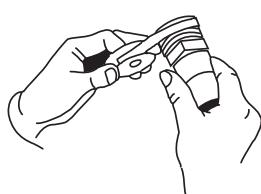
1. Apply pipe thread tape or sealant to the threaded end of both hose adapters.
