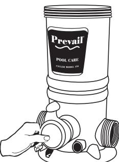
Carefully insert control dial back into housing.
