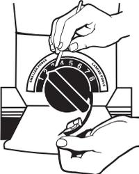
Using a small screwdriver or pointed tool to help guide it, make sure the snap ring stays in the groove as it is inserted.
