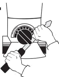
Using a large screwdriver, loosen the control dial. Carefully pry the dial until it pulls out.
