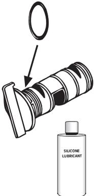
Carefully replace the rubber O-ring without stretching it. Apply silicone lubricant, that came with your POOL FROG Cycler, on O-ring.
