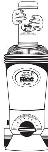
Line up the small leg of the POOL FROG Bac Pac with the small opening in the POOL FROG Mineral Reservoir and the large leg with the large opening. Lower POOL FROG Bac Pac into POOL FROG Mineral Reservoir until secure.
