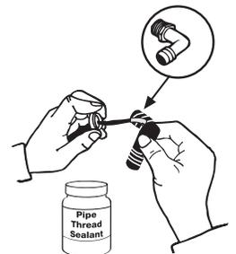
Following pipe thread sealant directions, brush sealant onto elbow threads.
