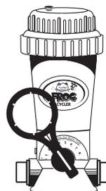
After each testing, adjust the dial up by 1/2 increment if the free chlorine reading has dropped below 0.5 ppm or adjust down by 1/2 increment if the reading has risen above 1.0 ppm. Continue this process each day until the free chlorine reading stabilizes to at least 0.5 ppm.
