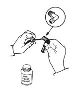
Following pipe thread sealant directions, brush sealant onto elbow threads.
