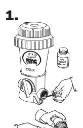
Following pipe thread sealant directions, brush sealant onto POOL FROG® threads in both ports and on both male adapters.
