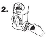
Screw a male adapter into each port of POOL FROG® Cycler and hand tighten.
