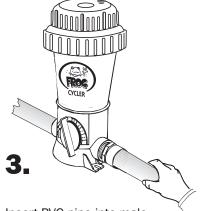
Insert PVC pipe into male adapters with a twisting action. Hold in place 5 to 10 seconds to bond.
