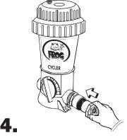
Insert reducer bushing into male adapter on both sides with a twisting action. Hold in place 5 to 10 seconds to bond.
