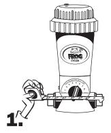
Measure the distance between POOL FROG® Cycler male adapters and cut out a section of pipe 3" less than that dimension.
