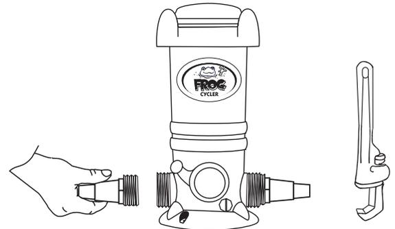
2. Screw adapters into each end of POOL FROG® Cycler. Hand tighten. Finish tightening by turning 1 to 2 revolutions with wrench. **DO NOT OVER TIGHTEN.**
