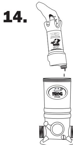
Lift FROG BAM® up and allow any water in the container to drain through the POOL FROG® Cyclor before discarding in trash.
