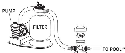
The POOL FROG® Cycler should always be installed between the filter and pool (or between heater and pool if applicable).
