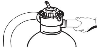
Screw one end of nipple into the filter return.
