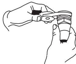
**4.** Apply pipe thread tape or sealant to threaded end of hose adapter.
