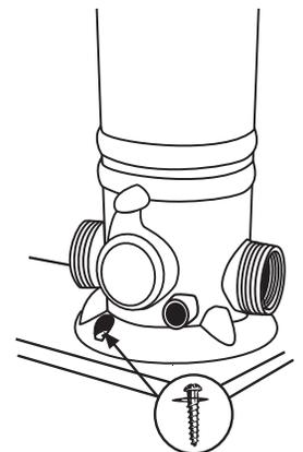
5. For better stability, POOL FROG® Cycler may be mounted on a base using Phillips pan head screws. One in front and two in back.
