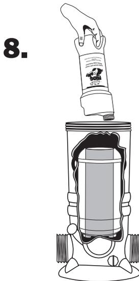
Insert upside down into center of POOL FROG® Mineral Reservoir pushing down firmly on key to puncture seal.
