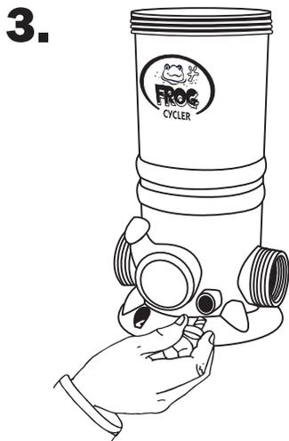
Unscrew knob from the front of POOL FROG® Cyclers. Allow all water to drain.
