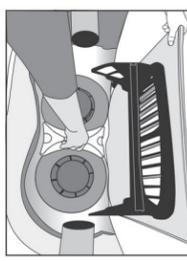
2. Hold weir door/filter plate out into the hot tub slightly or remove from hot tub. If cartridge holder is already installed between the filter cartridges, remove by pulling up on the handle.
