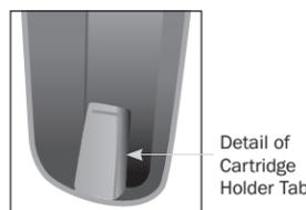
4. Then push the top part of the cartridge in until it snaps into place.
