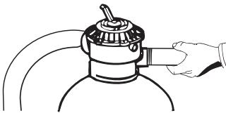
**2.** Screw one end of nipple into the filter return.
