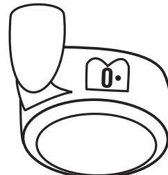
Turn off pump and turn dial to Setting 0. This reduces the flow of water into the unit when the cap is open.
