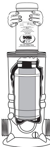
Line up the small leg of the POOL FROG® Bac Pac with the small opening in the POOL FROG® Mineral Reservoir and the large leg with the large opening. Lower POOL FROG® Bac Pac into POOL FROG® Mineral Reservoir until secure.
