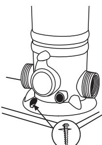
5. For better stability, POOL FROG® Cycler may be mounted on a base using Phillips pan head screws. One in front and two in back.
