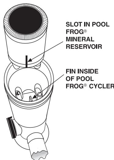
Find slot on side of POOL FROG® Mineral Reservoir and line up with fin inside the POOL FROG® Cycler. Lower POOL FROG® Mineral Reservoir into POOL FROG® Cycler until secure.
