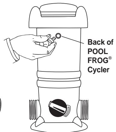
To replace, simply unscrew old knob and replace with the new one.
