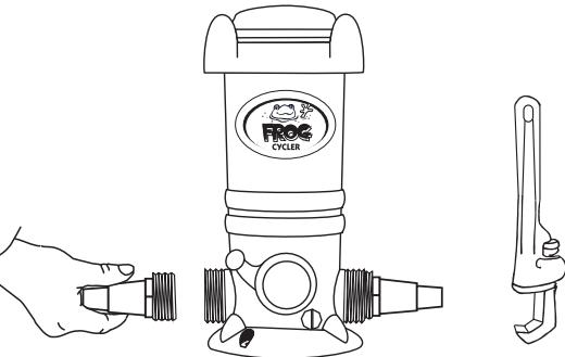
1. Apply pipe thread tape or sealant to the threaded end of both hose adapters.
