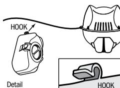
If only a small amount is left attach a new FROG @ease SmartChlor Cartridge and hook the old cartridge on the tether until it is completely empty.
