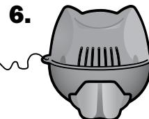
Replace the FROG @ease SmartChlor Cartridge when the system flips over and replace the complete FROG @ease Floating System that includes a FROG @ease Mineral Cartridge as directed under Step 2: Put the System to Work.
