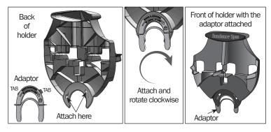
Installing the FROG @ease Cartridge Holder: With the filter cartridge in place, slide the holder down over the pipe where the nut is that holds the filter cartridge on.
