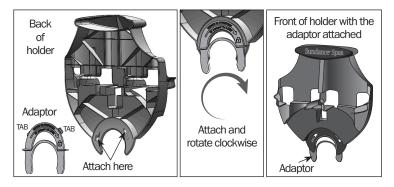
3. Installing the FROG @ease Cartridge Holder: With the filter cartridge in place, slide the holder down over the pipe where the nut is that holds the filter cartridge on.
