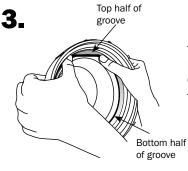
Roll your thumbs back and forth over the O-ring while pushing upward until the O-ring falls into the top of the groove.
