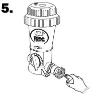
Screw elbow into reducer bushings on both sides.
