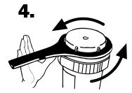
Open Pool FROG Cycler Cap. Use the cap tool included with Pool FROG Cycler to loosen cycler cap by hitting the handle with the flat of your hand counter clockwise.
