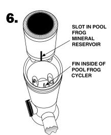
Find slot on side of Pool FROG Mineral Reservoir and line up with fin inside the Pool FROG Cycler.Lower Pool FROG Mineral Reservoir into Pool FROG Cycler until secure.
