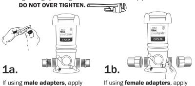
of using **male adapters**, apply pipe thread tape or sealant to the threaded end of each adapter.
