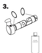
Replace both O-rings. Apply silicone lubricant that came with your FROG Pool Tender Cycler on O-rings.
