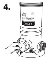
Carefully insert control dial back into housing.
