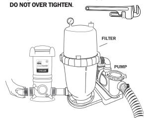
Attach return section of hose to the adapter with clamp. Tighten clamp with screwdriver.
