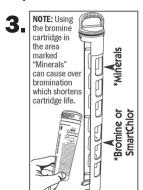
Snap the FROG Serene Mineral Cartridge into the area marked "Minerals" (top portion) and the FROG Serene Bromine Cartridge into the area marked "Bromine or SmartChlor" (bottom portion) making sure to line up the indentation at the top of the cartridges with the raised area on the holder.
