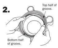
Place new O-ring in bottom half of groove.
