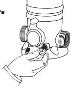
Unscrew knob from the front of Prevail Cycler. Allow all water to drain.
