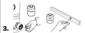
Following primer directions, brush primer on the inside of the adapters and to ends of pipe. Repeat this process with PVC cement following directions on that product.
