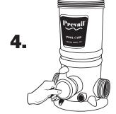
Carefully insert control dial back into housing.
