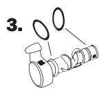
Replace both O-rings. Apply silicone lubricant that came with your Prevail Cycler on O-rings.
