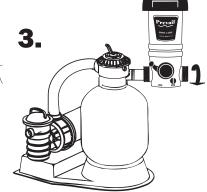
Screw either side of Prevail Cycler on to open nipple end until upright and secure.
