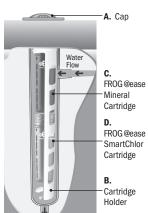
Cut-away view of cartridges snapped into holder and placed into the In-Line System.
