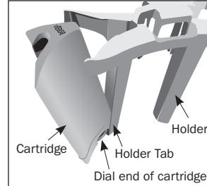
4. Then push the top part of the cartridge in until it snaps into place
