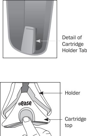
5. Follow the same procedure for the FROG @ease SmartChlor Cartridge into the other opening.
