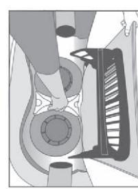
2. Hold weir door/filter plate out into the hot tub slightly or remove from hot tub. If cartridge holder is already installed between the filter cartridges, remove by pulling up on the handle.
