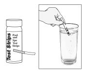
**5b.** Look at the **Total Alkalinity** reading first. Adjustments should be made to bring the Total Alkalinity in the range of **80 – 120 ppm** prior to making any adjustments to pH even if it throws pH off further.
