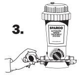
Measure the distance between the Sparco System male adapters and cut out a section of pipe 3" less than that dimension.
