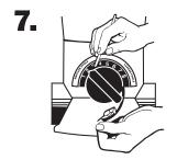
Using a small screwdriver or pointed tool to help guide it, make sure the snap ring stays in the groove as it is inserted.
