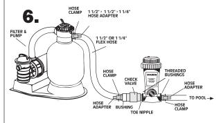
To prevent damage to heaters or filters, see your dealer about installing a **corrosion resistant check valve** which will reduce the back flow of chlorine gas when the Sparco System is turned off.
