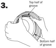
Roll your thumbs back and forth over the O-ring while pushing upward until the O-ring falls into the top of the groove.
