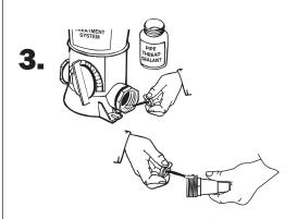
Apply sealant to threaded ends of both hose adapters and inside of both male adapters.
