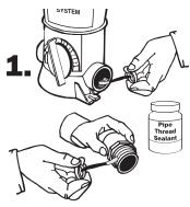
Following pipe thread sealant directions, brush sealant onto Sparco System threads in both ports and both male adapters.
