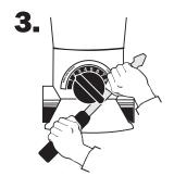
Using a large screwdriver, loosen the control dial. Carefully pry the dial until it pulls out.
