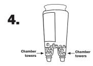
Invert Sparco Chamber and shake slightly until tablets fall into tower areas.
