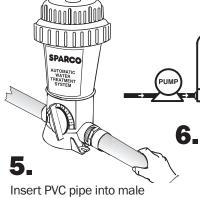
Insert PVC pipe into male adapters with a twisting action. Hold in place 5 to 10 seconds to bond.
