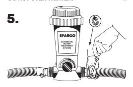
Attach the filter section of flex hose to one hose adapter and the return section of flex hose to the other hose adapter with clamps and tighten with screwdriver. Bi-flow valve design allows water flow in either direction.
