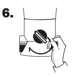
Insert the non-lipped end of snap ring into the groove opening beginning at the 5 o'clock position and push it up so that it threads itself around the control dial.
