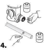
Following Primer directions, brush Primer on the inside of the male adapters and to ends of pipe. Repeat this process with PVC cement following manufacturer's directions on that product.
