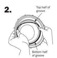
Place new O-ring in bottom half of groove.
