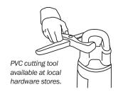
**3b.** Place curved section of tool around the narrow end of one Sparco Chamber tower and line up blade on indent
