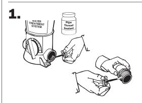
Following pipe thread sealant directions, brush sealant on to Sparco System threads in both ports and both male adapters.
