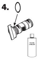
Carefully replace the rubber O-ring without stretching it. Apply silicone lubricant that came with your Sparco System on O-ring.
