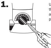
Using a needle nose pliers, find the snap ring tail located at approximately the five o'clock position under the control dial.
