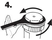
**Open POOL FROG Cycler** Cap. Use the cap tool included with POOL FROG Cycler to loosen cycler cap by hitting the handle with the flat of your hand counter clockwise.
