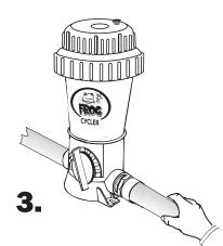
Insert PVC pipe into adapters with a twisting action. Hold in place 5 to 10 seconds to bond.
