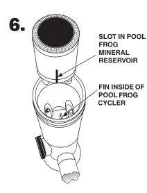
Find slot on side of POOL FROG Mineral Reservoir and line up with fin inside the POOL FROG Cycler. Lower POOL FROG Mineral Reservoir into POOL FROG Cycler until secure.
