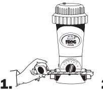
Measure the distance between the outside adapters and cut out a section of pipe 3" less than that dimension.
