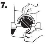
Using a small screwdriver or pointed tool to help guide it, make sure the snap ring stays in the groove as it is inserted.
