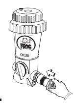
Insert reducer bushing into male adapter on both sides with a twisting action. Hold in place 5 to 10 seconds to bond.
