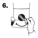
Insert the non-lipped end of snap ring into the groove opening beginning at the 5 o'clock position and push it up so that it threads itself around the control dial.
