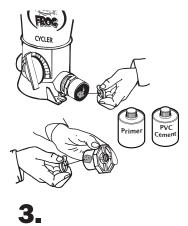
Following Primer directions, brush Primer on reducer bushings and inside of male adapters. Repeat this process with PVC cement following manufacturer's directions on that product.
