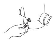
Unscrew knob in the back of POOL FROG Cycler. Allow all water to drain.
