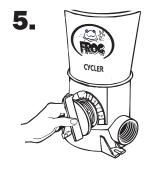
Push control dial completely into the housing and turn the dial to setting 2.
