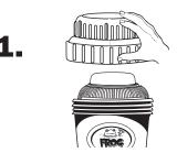
Turn pump off. Turn control dial to Pac Removal. Remove cap from POOL FROG Cycler and stand back to let any chlorine fumes dissipate.
