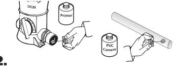
Following Primer directions, brush Primer on the inside of the adapters and to ends of pipe. Repeat this process with PVC cement following manufacturer's directions on that product.
