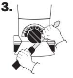
Using a large screwdriver, loosen the control dial. Carefully pry the dial until it pulls out.
