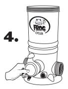
Carefully insert control dial back into housing.
