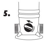
Replace locking pin by pushing it through the slots on the dial until it locks into place.
