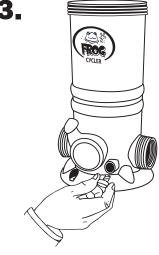
Unscrew knob from the front of POOL FROG® Cycler. Allow all water to drain.
