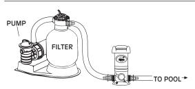
The POOL FROG® Cycler should always be installed between the filter and pool (or between heater and pool if applicable).
