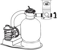
Screw either side of POOL FROG® Cycler on to open nipple end until upright and secure.
