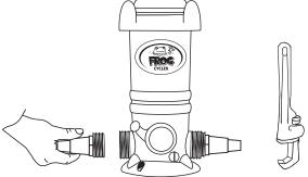
Screw adapters into each end of POOL FROG® Cycler. Hand tighten. Finish tightening by turning 1 to 2 revolutions with wrench. DO NOT OVER TIGHTEN.
