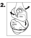
Align the chlorine cartridge with tab guides on the mineral cartridge. Push together until you hear the cartridge click into place.
