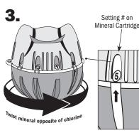
Twist the mineral cartridge opposite of the chlorine cartridge until the setting number for your pool size is lined up with the arrow. Even at the lowest possible setting of 0 there will be some chlorine released into the pool.
