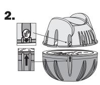
Line up arrow on chlorine cartridge with the unlock symbol on the mineral cartridge. Push together and twist to lock.
