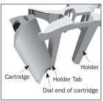
Then push the top part of the cartridge in until it snaps into place
